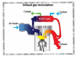
Since EGR reduces the available oxygen in the cylinder, the production of PM increases when EGR is applied. NOx and PM are traded against each other in many aspects of diesel engine design. Very high temperatures in the combustion chamber help reduce the emission of soot but produce higher levels of NOx gases. Lowering the peak temperature in the combustion chamber reduces the amount of NOx produced but increases the likelihood of soot formation.
