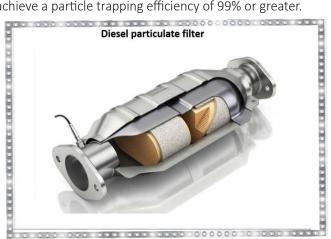
The honeycomb design provides a large filtration area while minimising pressure losses, and has become the standard, so-called wall-flow filter for most diesel exhaust filtration applications. Ceramic materials are widely used for particulate filters, given their good thermal durability, with the most common ceramic materials being cordierite, silicon carbide, and aluminium titanate.
