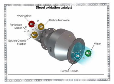
The DOC also protects the DPF. Hydrocarbon liquids or vapor can interfere with the DPF's ability to trap and remove particulate matter, so engine manufacturers often route the exhaust through the DOC first, then into the DPF.
