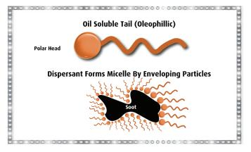
As already discussed, the EGR system recirculates a small amount of cooled exhaust gas back into the combustion chamber which lowers the combustion temperature, which in turn reduces the NOx gases. However, recirculating exhaust gas also creates a multi-pass opportunity for soot to accumulate in the engine oil.
