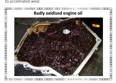
The use of EGR systems can increase the rate at which the oil oxidises as many of these systems rely on the engine's coolant system to reduce exhaust gas temperatures, which increases the engine running temperature. This elevates the engine oil sump temperature, which in turn puts more demand on the lubricating properties of the oil. Exacerbating the situation is the added requirement of increased oil drain intervals, which means the oil needs to be in use for longer.
