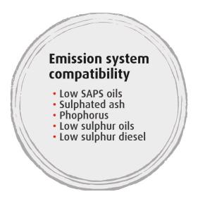
Unfortunately, these chemicals are proving problematic with the current emission technology on offer and, as a result of these compatibility issues, lubricant manufacturers are facing chemical restrictions which are aimed at protecting emission control systems by limiting the levels of these chemicals used to formulate a lubricant.
