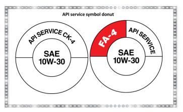
The API FA-4 fuel efficiency category requires lubricants to pass the same performance tests as API CK-4, with the addition of a HTHS viscosity limit of between 2.9 and 3.2cP, to deliver increased fuel efficiency benefits whilst maintaining engine
