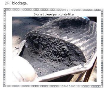
The ash can occupy a large portion of the filter volume, as it may accumulate in a thin layer along the channel walls or pack in plugs towards the back of the filter channels.
