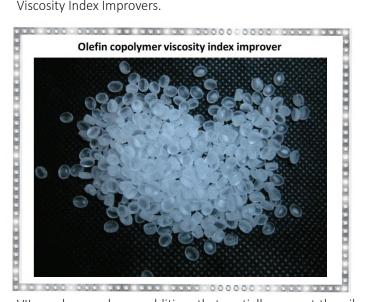
VIIs are large polymer additives that partially prevent the oil from thinning out (losing viscosity) as operating temperatures increase. They are also responsible for better oil flow at low temperatures, resulting in reduced wear. VIIs contribute to improved fuel economy primarily through shear thinning and viscosity temperature properties.
